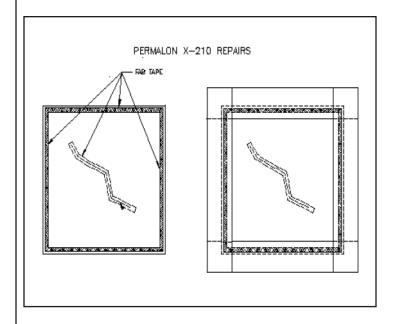
Small rips and tears in the liner can be repaired with Fab Tape™ and a small Permalon® patch.
