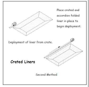
The second method is preferred as 1) Potential for damage to the liner is minimized, and 2) Heavy equipment can be used to aid in the removal of the liner from the crate.
