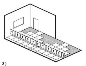
Loose lay the tiles (without adhesive) starting along the centrelines and following the arrows printed on the back of the tiles taking special care to the alignment of joints and/or pattern.
